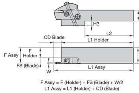
$F \text{ Assy} = F \text{ (Holder)} + FS \text{ (Blade)} + W/2$
