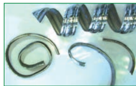
Material steel ST52; Insert size 6mm; f = 0,25 mm/U
