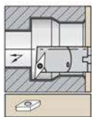
Steel shank with through coolant.
